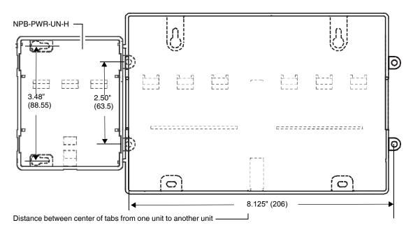
Fig. 14. WEB/CP-700 with power supply attached.
